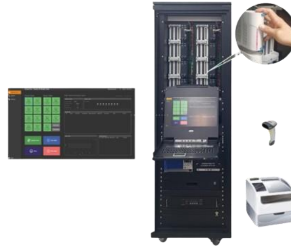
DCS I/o Module & Relay Diagnosis Equipment
